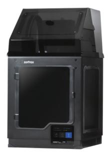
HEPA Cover is a filtering device designed to intercept UFPs and unpleasant odors released in the 3D printing process. It also keeps the temperature in the printing chamber stable to reduce warping and shrinkage.
