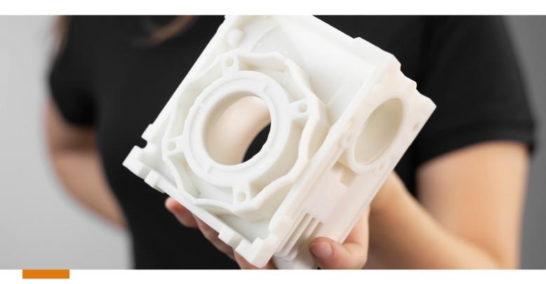
**WORM GEARBOX REDUCER.** A worm gear reducer is one type of reduction gear box generally used to take a rated motor speed and produce a low speed output with higher torque value based on the reduction ratio. Designers can test the ratio of speed reduction as well as the torque output multiplier to achieve the best results.
