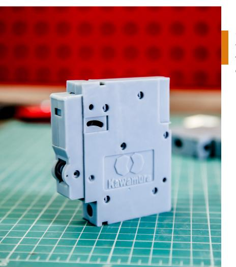
**GFCI CASING.** A casing for the ground fault circuit interrupter (GFCI) made for testing to prevent serious harm from an ongoing electric shock.
