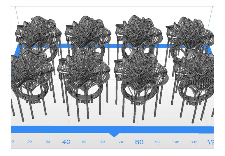
Regardless of whether one or multiple rings are projected onto the platform, the printing speed remains the same.
